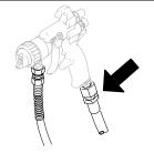
**3**Connect the fluid hose to the sprayer. Tighten securely. 將液流軟管連接到噴塗機上。連接要牢固。
