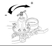
2. Adjust fluid pressure so stream from gun travels 6-8 in. straight before falling off.
