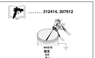
**9.** Remove the suction tube from the solvent. Continue to spray until all solvent is out of the gun.
